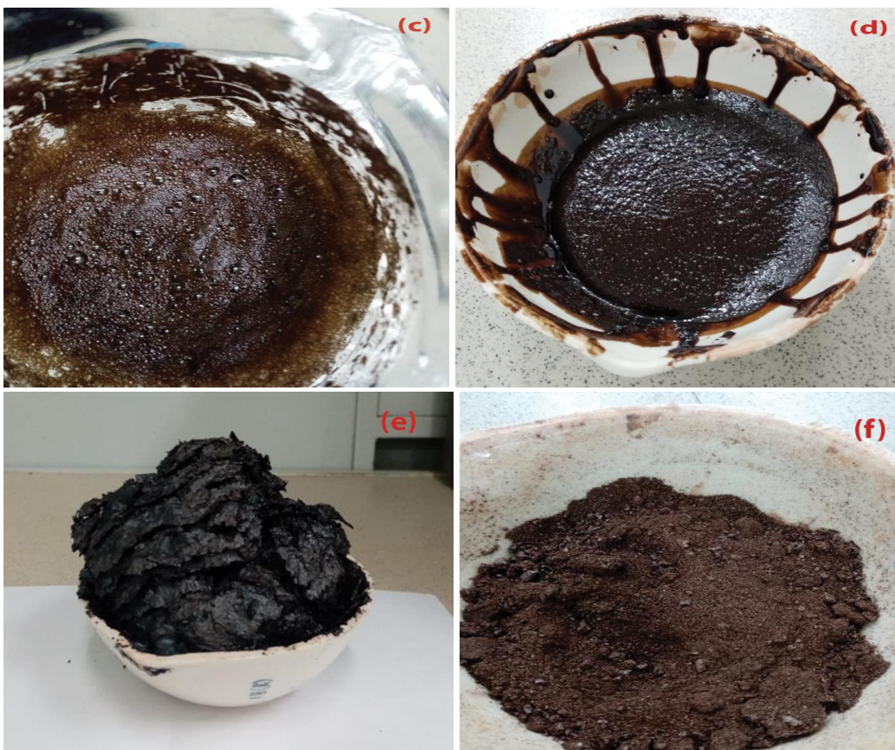
Figure 2.5 – Synthesis of \text{Ni}_{0.5}\text{Zn}_{0.5}\text{Fe}_2\text{O}_4 nanoparticles by citrate precursor method: (a) the metal salts aqueous solution in the flask, (b) using \text{NH}_4\text{OH} to maintain the pH of the solution at 7, (c) heating the solution at 90^\circ\text{C} for 6 h, (d) formation the viscous gel, (e) formation a fluffy carbonaceous pyrolyzed mass and (f) obtaining nanoparticles ferrite
