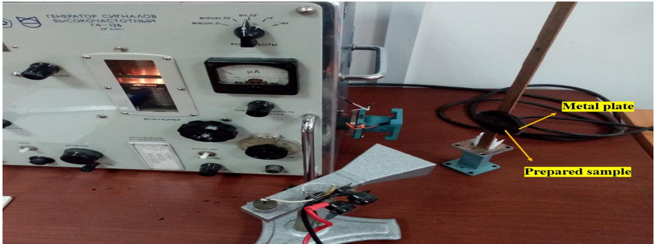
Figure 2.3 – Experimental setup for measuring the reflected power of the EM waves for the microwave absorption model
