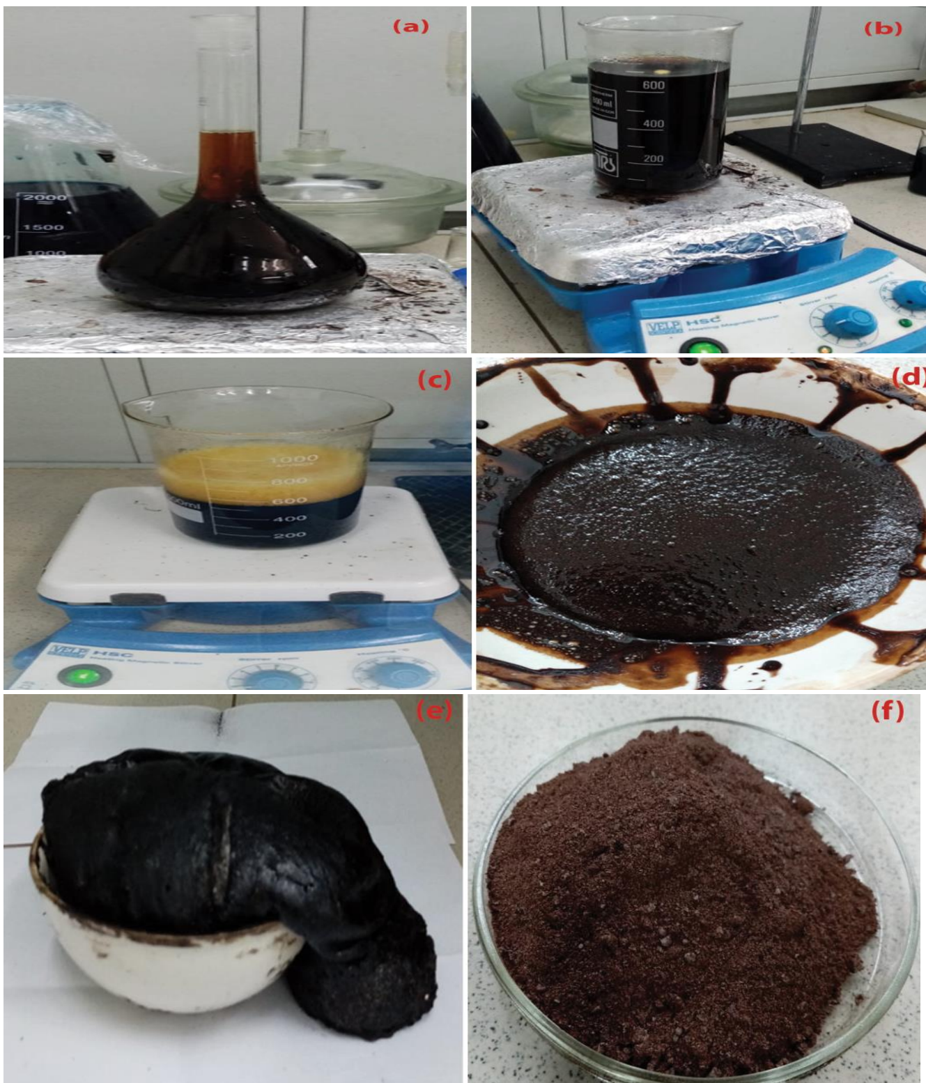
Figure 2.7 – Synthesis of NiZn ferrite nanoparticles by self-combustion method: (a) the metal salts aqueous solution in the flask, (b) blending the whole mixture, (c) heating the solution at 90 °C, (d) formation of a viscous liquid, (e) formation a fluffy carbonaceous pyrolyzed mass, and (f) obtaining nanoparticles ferrite
